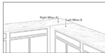
Eliminate hours from the typical installation process with Stretta's quick and simple step-by-step install process. Simply join Right Miter-A and Left Miter-B to form a 90-degree angle - saving you time & money.
