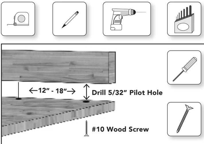
CenterPointe backsplash material may be screwed to the CenterPointe butcher block countertop prior to installation by drilling pilot holes and screwing from the bottom of the block into the backsplash material. Attachment to the cabinet base is not necessary for the attachment of the backsplash. The number of installation fasteners is to be determined by the installer. It is recommended that fasteners be put every 12"-18".
