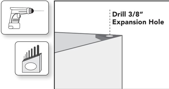
Use a 3/8" drill bit to create an expansion hole in the corner block cabinet base in the same location as the pilot holes in step 4, repeat for each fastener. This will enlarge the pilot holes in the sub-top created with the 5/32" bit. DO NOT enlarge the pilot holes in the CenterPointe countertop.
