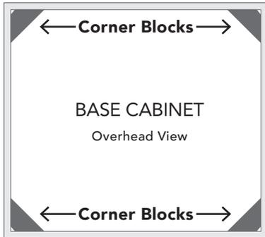
Minimal screws are required as the top will be held down by self-weight. Use only enough screw to secure the countertop. Too many screws can keep the top from moving freely and can result in damage. Most cabinet manufacturers provide corner blocks or plywood within the cabinet for attaching the countertop to the cabinet base; screw locations are usually in the corners. The number of screws is to be determined by the installer. It is recommended to apply screws every 12 to 18 inches.
