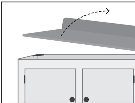
It is not recommended to attach your CenterPointe countertop directly on top of a solid underlayment or existing countertop; remove existing top if applicable.
