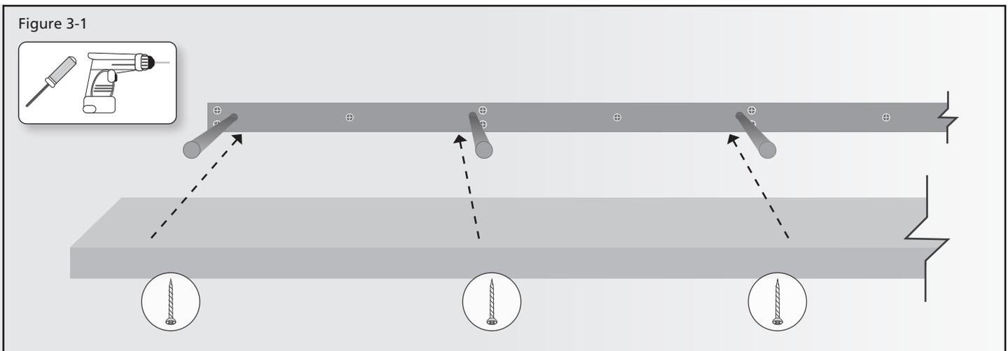
Align the mounting bracket with the pre-drilled holes on the back side of the shelf and slide into place. Locate the 1-1/8 inch finishing screws and using a drill, screw them into the pre-drilled holes on the face of the shelf (Figure 3-1). Repeat process with additional shelves.
